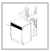
1. The end of the tube should be directed downwards, to prevent warm moist air from condensing in the room or in the dryer.
